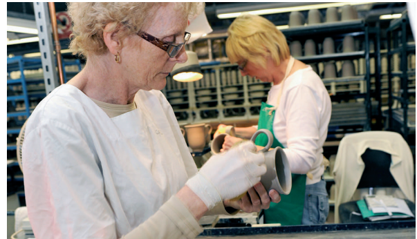
Pictured: Product being sponged in the cup-making department of our UK manufacturing plant.
