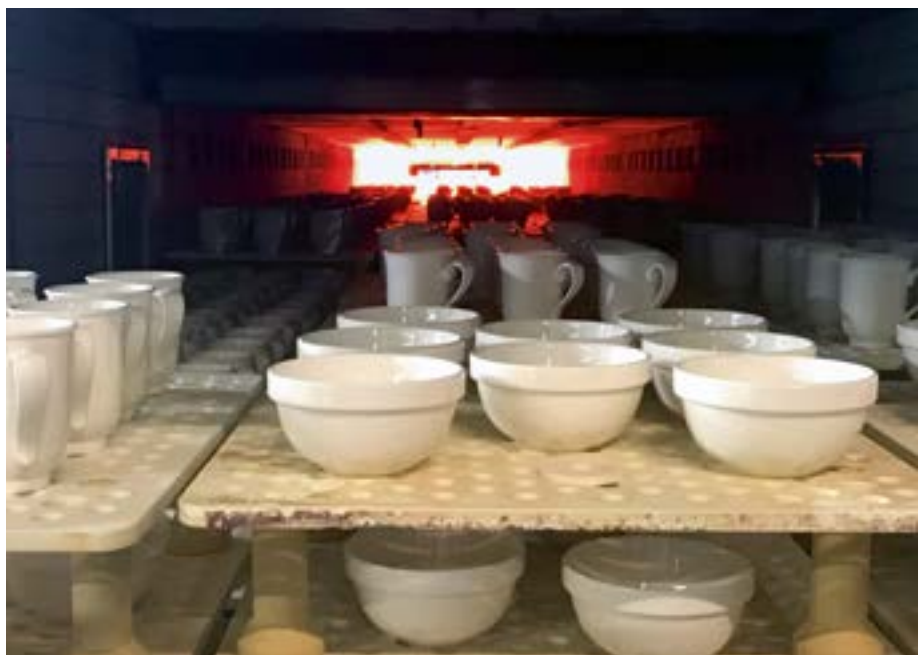
Pictured: Portmeirion UK has reduced firing temperatures on its glost kilns.
